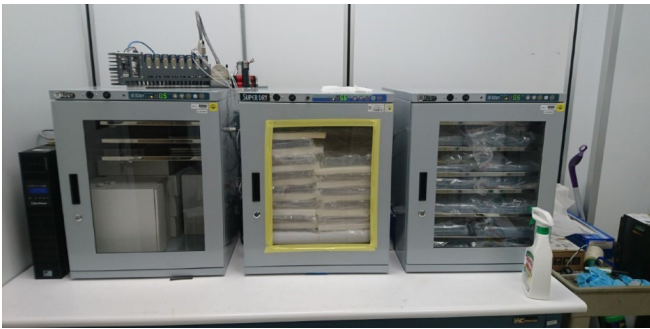
FIG. 1. Three XDry dry boxes containing 43 aerogel tiles. The cRIO used for monitoring is on top of the left-most dry box.
